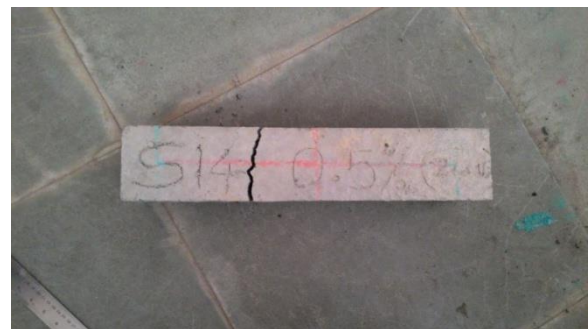
Fig.5. Specimen after flexural strength test
