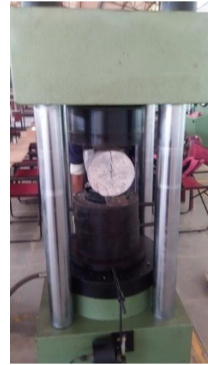
Fig.4. Split tensile strength testing
