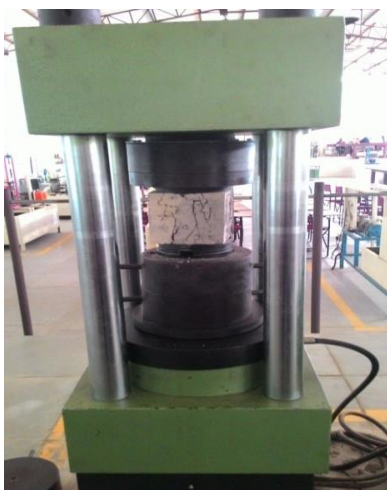
Fig.3. Compressive strength testing
