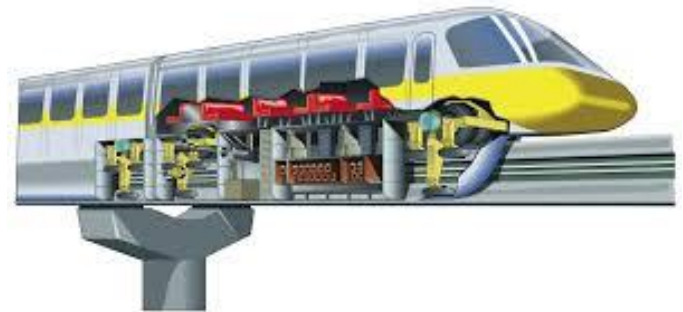
Fig. 3. Sectional view of straddle type monorail
