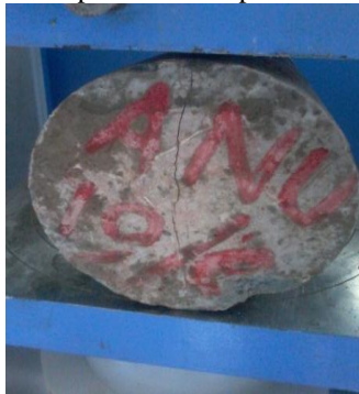
Fig 5: Determination of split tensile strength of cylinder
