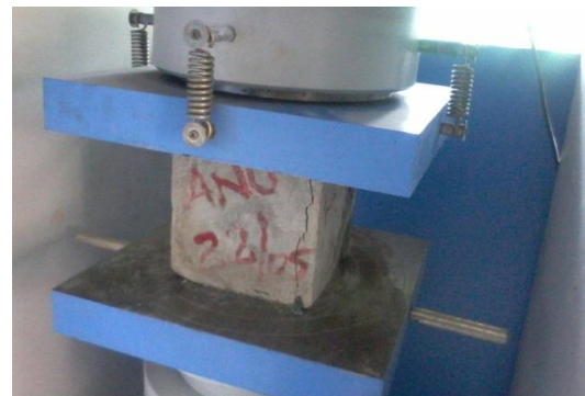
Fig 3: Compression test of concrete cube
