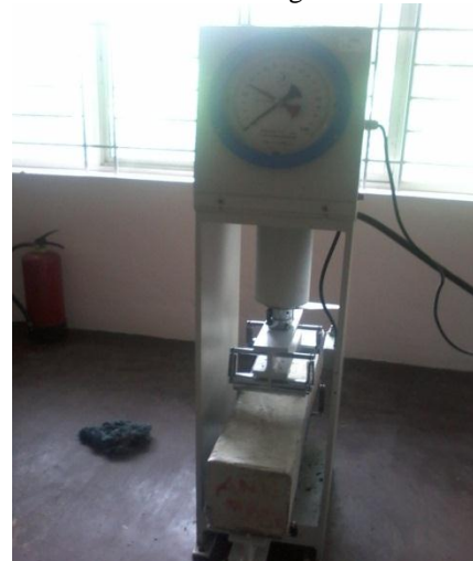
Fig 4: Determination of flexural strength of beam
