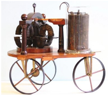
Fig.10. The first electric horseless carriage [24, 29]
