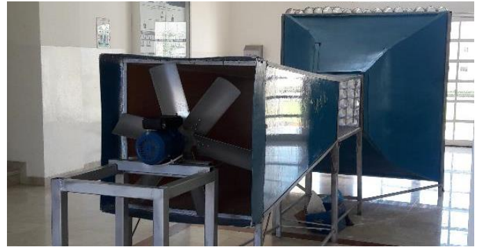
Fig. 6.1 Newly built subsonic wind tunnel in IBRICT.
