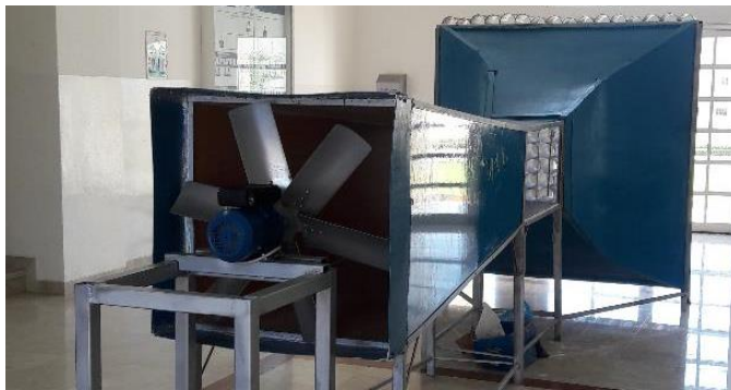
Fig. 6.1 Newly built subsonic wind tunnel in IBRICT.
