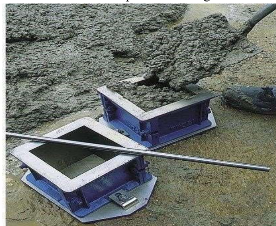
Fig.3. Filling mortar in Moulds
