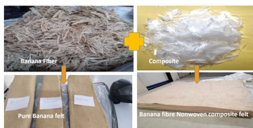
Fig. 3. The manufacturing process of nonwoven composite felt
