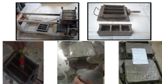
Fig (2): Different steps are involved in sample preparation.
