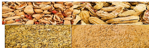
Fig (1): Peanut shells before and after cleaning, and their powder after crushing.
