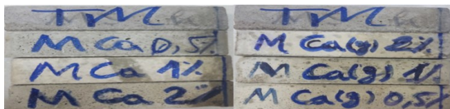
Fig (3): Different samples of fine (M Ca) and slightly coarser (M Ca(g)) peanut shell powder.
