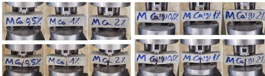
Fig (4): The images represent flexural strength testing (three-point bending)
