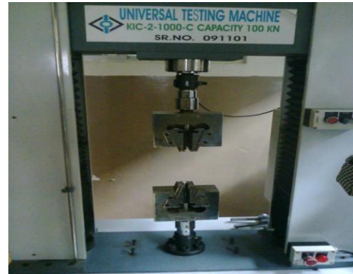
Fig4: Tensile test in Universal testing Machine
