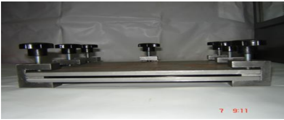
Fig 2: Assembly of mold used to fabricate composites
