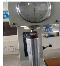
Fig 8: Specimen mounted on Rockwell hardness test machine
