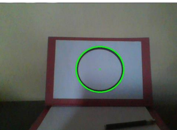
Fig.7 Center and circle on image frame using Hough circle transform
