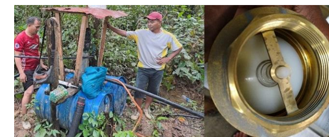
Fig. 3: The left image shows the blue and black bags that were used to carry the tools and the cylindrical black plastic at the bottom was used to bring long screwdrivers. The right image is the one way valve is the intake point within the river
