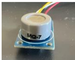
Fig. 2. MQ7 Sensor detects H2 and CO gases
