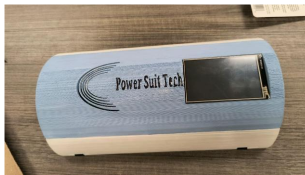
Fig. 13. The top of the EVE Sleeve: Nextion HMI display and 3D printed case
