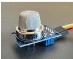
Fig. 1. MQ6 Sensor detects LPG and CH4 gases
