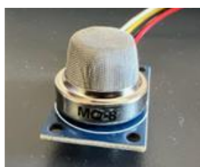
Fig. 4. MQ8 Sensor detects H2 gas
