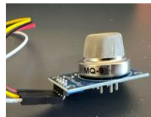
Fig. 5. MQ9 Sensor detects LPG and CO gases
