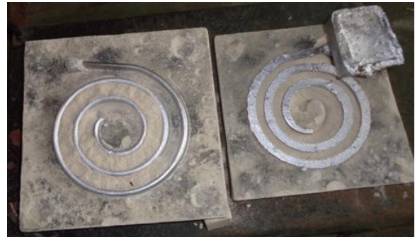
Fig.4. The outcome of the alloy's fluidity when it is solidified
