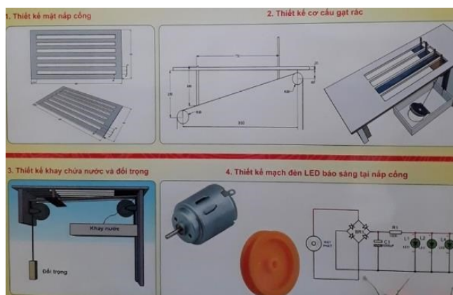
Fig. 3. Self-cleaning drain cover (10)
