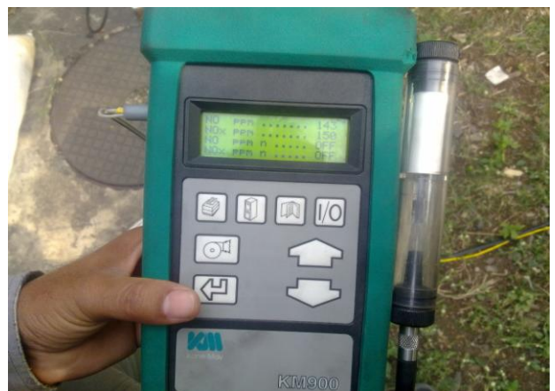
Fig. 6 Exhaust Gas Analyzer
