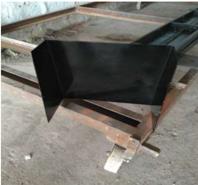
Fig 8: Cessna 152 aircraft upper cowling with GLARE Coating
