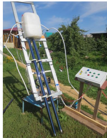
Fig. 2. Photo of solar desalination plant
