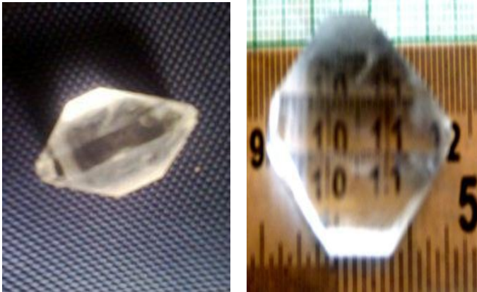
Fig. 1: 0.2 wt % L-alanine doped KDP crystal
