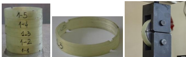
a) Prepared composite test ring b) split disc fixture
