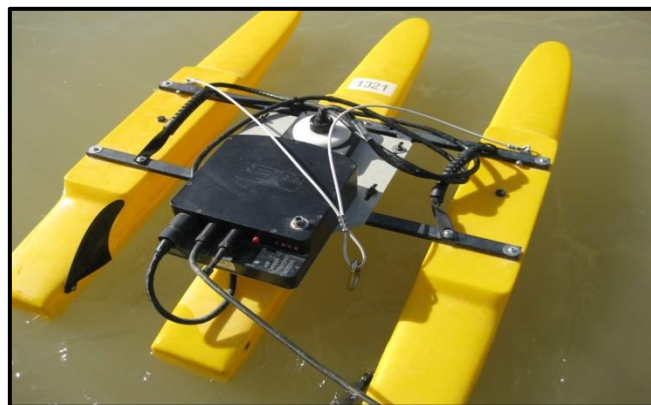
Fig. 3: SonTek River Surveyor ADCP
