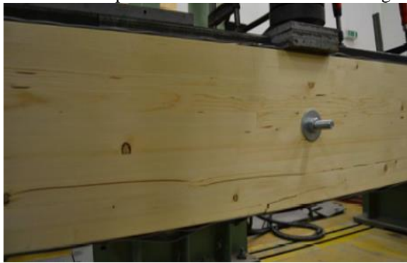
Figure 10: Failure pattern under ultimate load C1-GL-N
