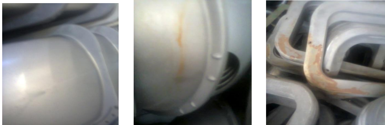
Figure 1 represents defects such as black marks, Very light yellow marks, Marks of rust.
