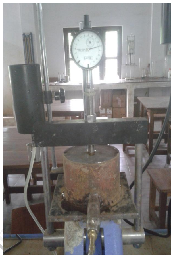
Fig 5. Consolidation test performed in laboratory using the new mould
