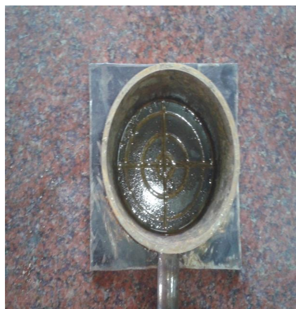
Fig 3. Top view of mould in which sand compaction piles are modeled
