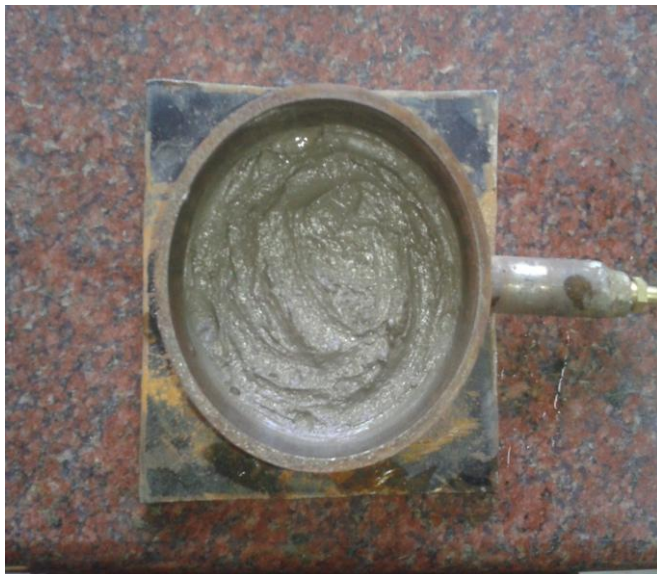
Fig.4.Sand bed prepared for providing sand compaction piles
