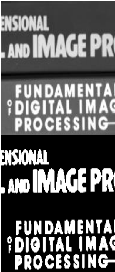
Figure 2: Gray scale image, Binary image after Erosion by 2x2 square elements structure
