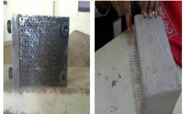
Fig.3.a) Mould with perforations b) Optical fiber embedded in the sample
