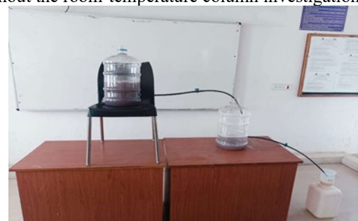
Fig- 4.6: Experimental Setup for Column study
