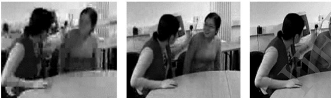
Fig 3. A video frame compressed at the same bitrate using MPEG-2 (left), MPEG-4 Visual (center) and H.264 compression (right) [13].
