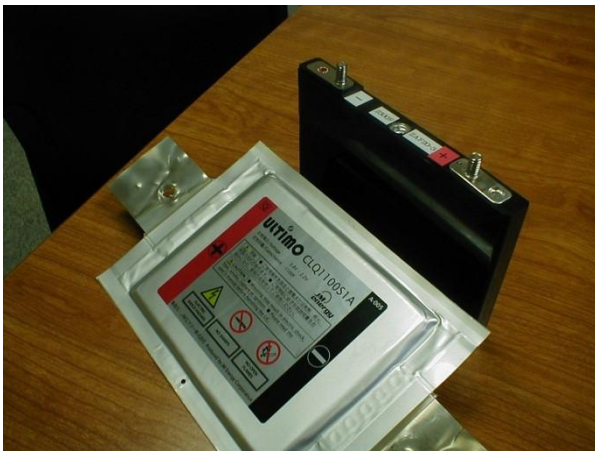
Fig-2 Photographs of the JSR Micro 1100F and 2300F devices
