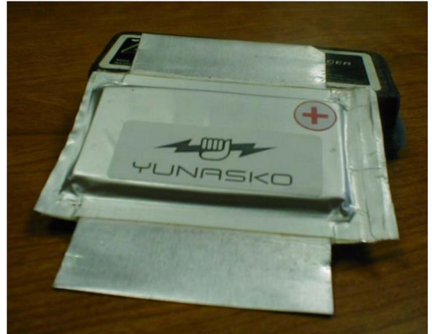
Fig-3 Photograph of the 5000F Yunasko hybrid ultracapacitor device
