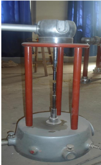
Fig. 3. Two cylindrical electrode with a diameter of 25mm used in dielectric strength test in high voltage laboratory.
