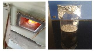
This product is treated with Concentrated HCl solution. And acid solution is taken on the basis of, for 1 gram Mg 50ml Hcl. After adding HCl, the MgO and MgSi converts into  $MgCl_2$  and it is AN exothermic reaction. Reactions occurred in solution are following
