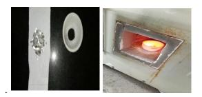
Both the samples are collected in a crucible and placed in electric muffle furnace until the magnesium burns and react with the sand. Normalizing of sample was done by cooling them in presence of air after heat treatment. During heat treatment
