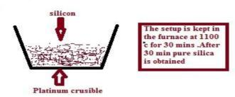
The silicon product was placed in a platinum crucible weighed. The setup is put in a furnace at 1100 <sup>0</sup>c for 30 minutes. After which it was removed allowed to cool in a desiccators and weighed again. Pure silica is obtained in this process.
