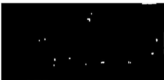
Fig. 17. Vehicle detection result using grayscale morphological operation on dark background image
