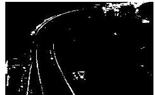
Fig. 14. A grayscale light background frame after thresholding using the Otsu's method
