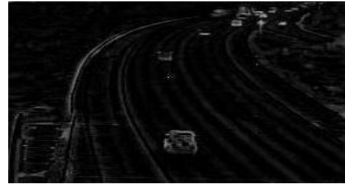
Fig. 11. A grayscale top-hat transformed frame
