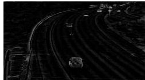
Fig. 13. A grayscale bot-hat transformed frame
