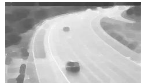
Fig. 12. A grayscale closing transformed frame
