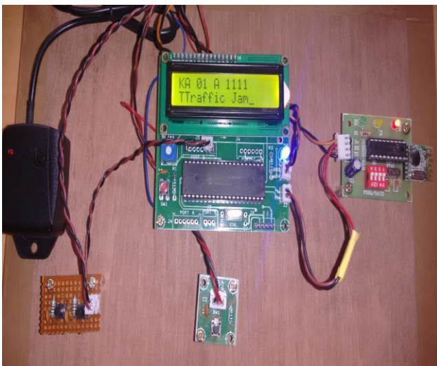
Figure 12: Result on hardware showing that the traffic jam has occurred and from which vehicle the message was generated.
