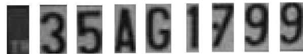
Figure 8. Character bitmaps as small image data set found as a result of the segmentation phase
