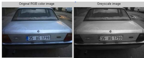
Figure 2. Car image conversion from rgb scale to greyscale for further feature extraction process
