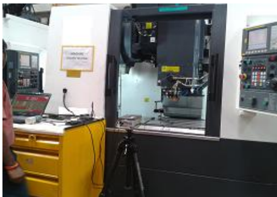
Figure 2: Laser interferometry setup
