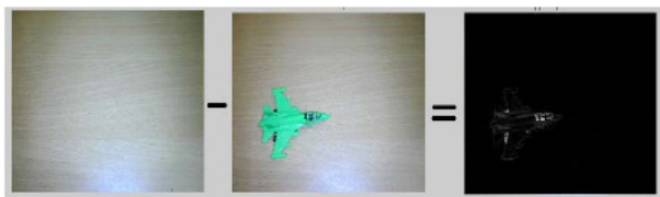
Fig 3. Subtraction of image captured by camera from background image to segment/detect intruding object.
