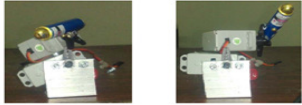
Fig 9 Servo motors mechanism for decoding angle of projectile launch
