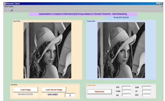
Figure 5: The cover image and the watermarked image after embedding.
