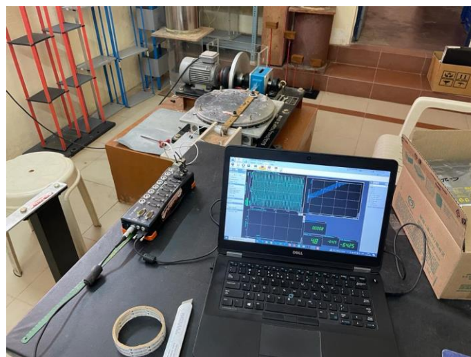
Photo 6.4: Oscillator connected to Data Acquisition System & Computer
