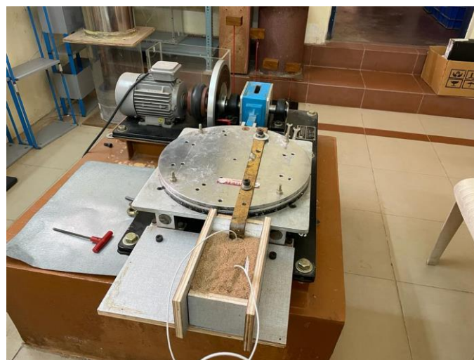
Photo 6.2: Oscillator arrangement attached to shaking table & box filled with Soil.
