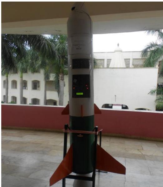
Fig. 7.3 Weather module mounted in a model rocket
