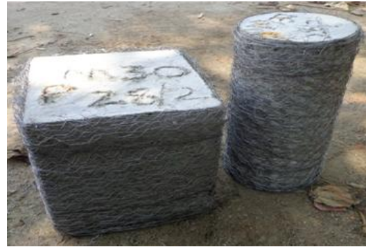
Figure.2.View of Cubes and Cylinders Wound with Wire Mesh
