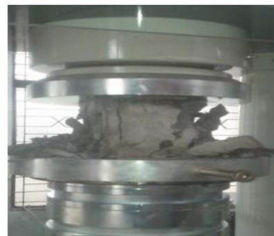
Figure.4.View of Cubical Specimen at Failure under Ultimate Loading
