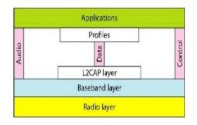
1) Radio Layer: The radio layer is roughly equivalent to the physical layer of the Internet model. Bluetooth devices are low-power and have a range of 10 m.
