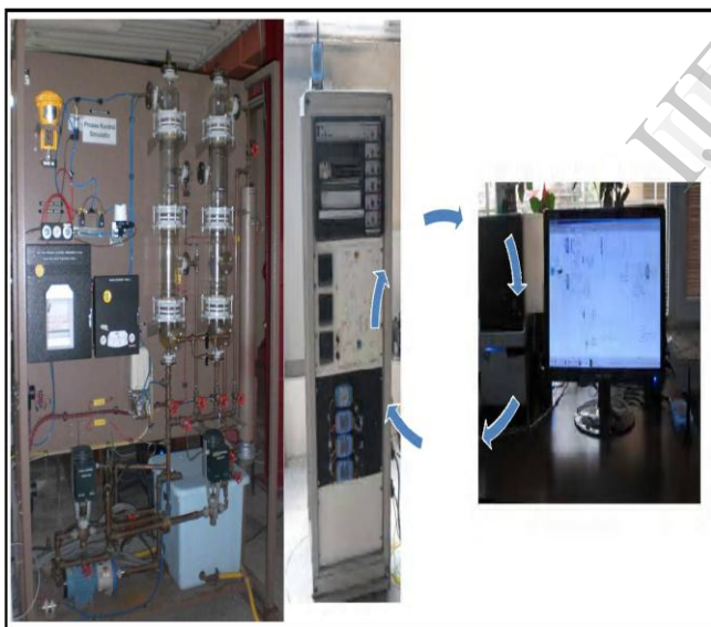
Figure 1. Experimental system: Process simulator, control panel and computer on-line connected to simulator with wireless technology
