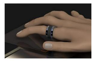
When the user switches ON the Pureth Pointer, the device automatically connects to the computer via Bluetooth. Now the Pureth Pointer senses the motion of the finger. The way the user moves the finger, the same way the cursor on the screen moves. The Pureth Pointer not just control cursor but does other task by following 4 touch inputs.
