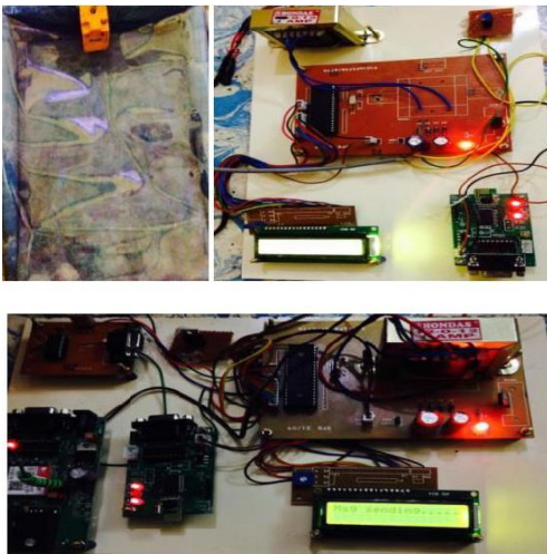
Figure 10. Prototype Model Output For Abnormal Pressure When Value Is Greater Than 400
