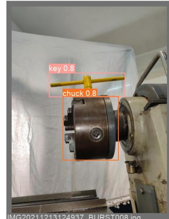
Figure 9: Test result indicates the detection of chuck and chuck key
