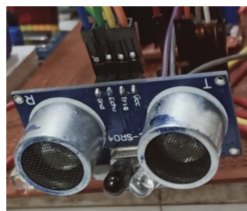
Fig. 12. Ultrasonic and IR sensor
